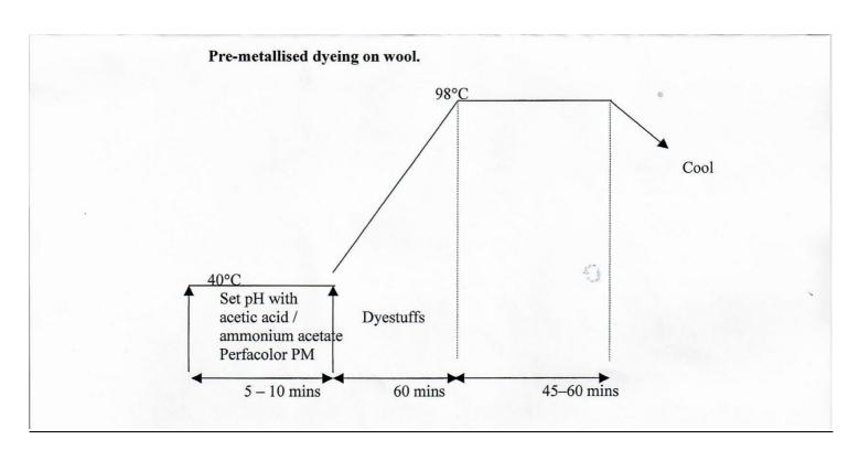
When making additions it is advisable to pre-mix the dyestuff with the **Perfacolor PM** at the correct temperature, which can be from 75°C-100°C, depending on the machine and the dyestuffs in use.
